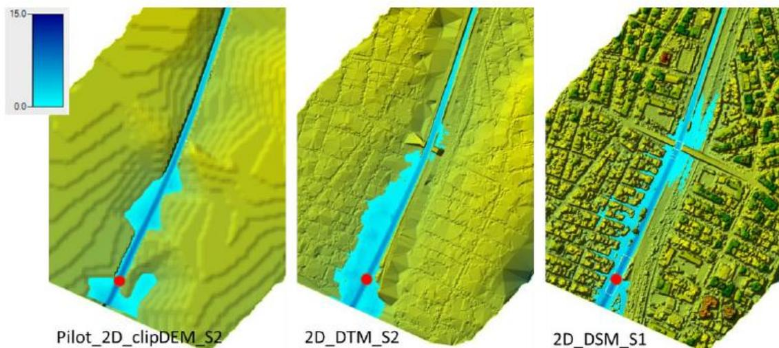
Figure 17: Inundation at the downstream part of three models: original Digital Elevation Model, drone Digital Terrain Model and drone Digital Surface Model. Source: Phuoc (2019).
