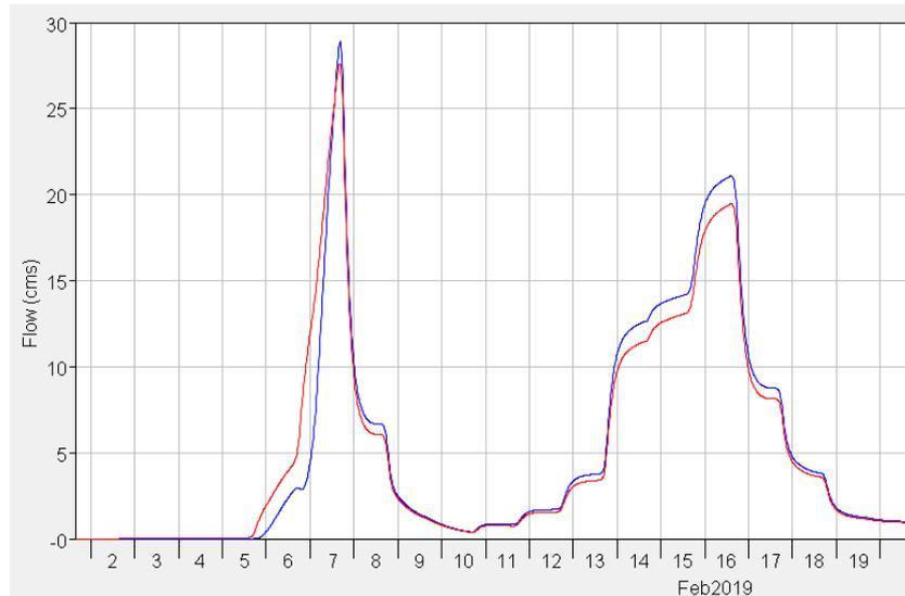
Figure 16: Discharge hydrographs for Kifisos hydrological model. Red line represents the discharge with the outdated CORINE land cover, while the blue line represents the model with the updated land cover.
